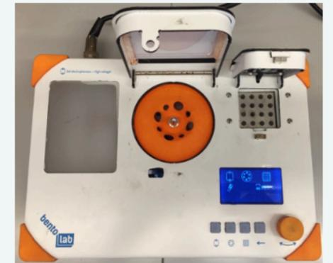
The Bento lab is a miniature lab with a centrifuge, thermocycler and an electrophoresis compartment.
